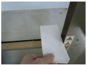
② Once the START switch is pressed, the tape is tightened, glued, and cut, and banding is completed.
