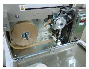
⑤ Insert the tape end into the tape guide, pass the tape until it touches the rubber roller, then lightly put a hand on the arrow, and hold the tape.
