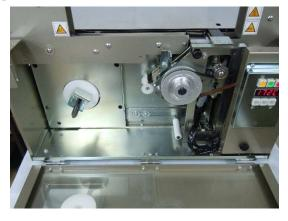
3 Place a tape on the paper tube holder. \*Be careful with the direction of the tape.
